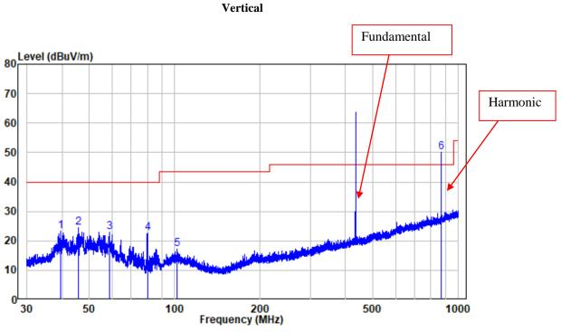
Site : chamber Condition: 3m VERTICAL Job No. : SZNS1220812-36596E-RF Test Mode: Transmitting
