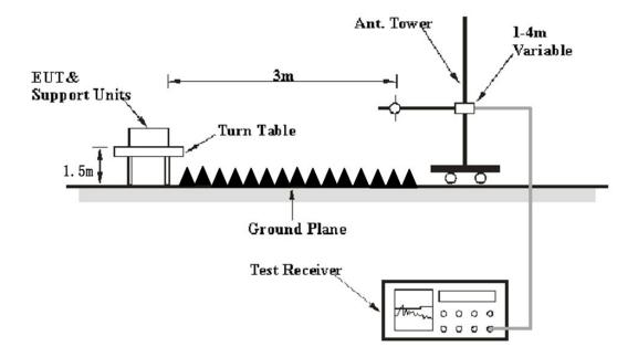
The radiated emission tests were performed in the 3 meters test site, using the setup accordance with the ANSI C63.10 - 2013. The specification used was the FCC 15 § 15.209, 15.205 and 15.231.
