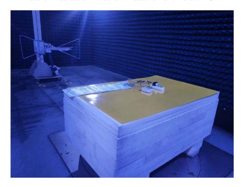
Photo of Radiated Emission Measurement Above 1GHz
