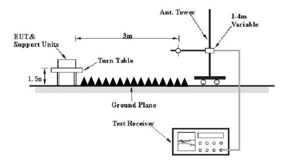
The radiated emission tests were performed in the 3 meters test site, using the setup accordance with the ANSI C63.10 - 2013. The specification used was the FCC § 15.209, 15.205 and 15.231.
