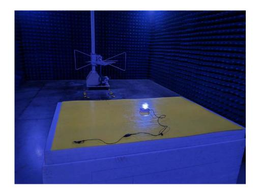
Photo of Radiated Emission Measurement Above 1GHz
