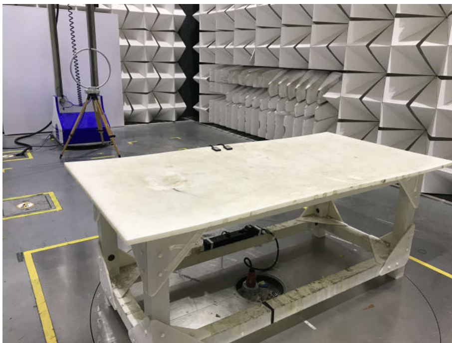
Radiated spurious emission Test Setup-2 (Below 30M)
