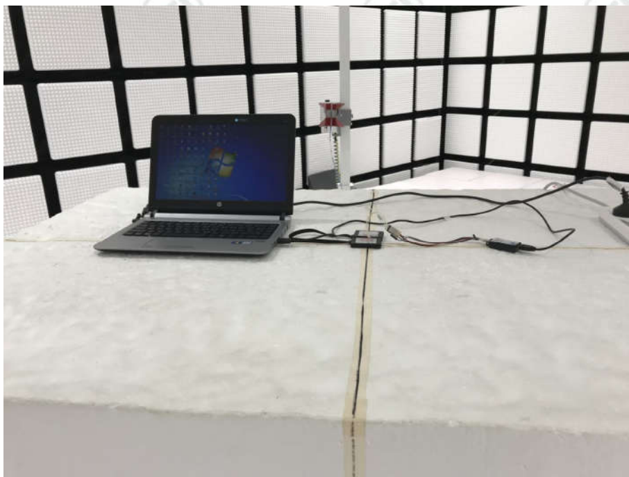
Radiated spurious emission Test Setup-3 (Above 1GHz)
