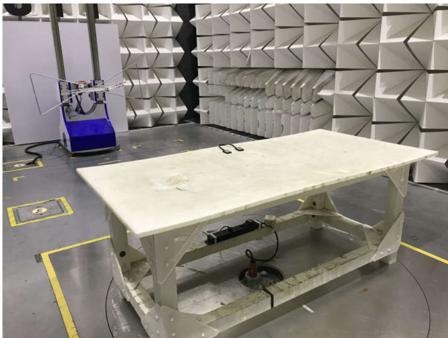
Radiated spurious emission Test Setup-1 (Below 1GHz)
