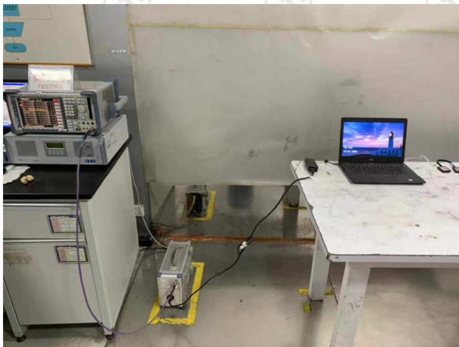
AC Conducted Emissions Test Setup
