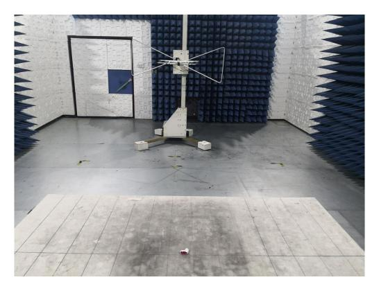
RADIATED EMISSION TEST SETUP ABOVE 1GHZ
