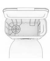
2. Wipe the transmitter window clean, making sure it is not blocked or covered.
