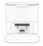
4. Unplug the station. Inspect the disposal vent and air pathway. Clean and remove any congestion.
