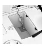
3. Slide the new battery into UltraVision.
