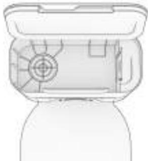
4. Unplug the station. Inspect the disposal vent and air pathway. Clean and remove any congestion.
