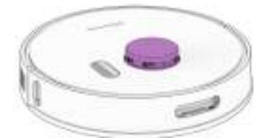
**Important Note:** Orb-i's SLAM LiDAR is a sensitive sensor. Do not apply force, insert objects, or adjust the SLAM LiDAR. Do not sit on Orb-i or place items on top of him.
