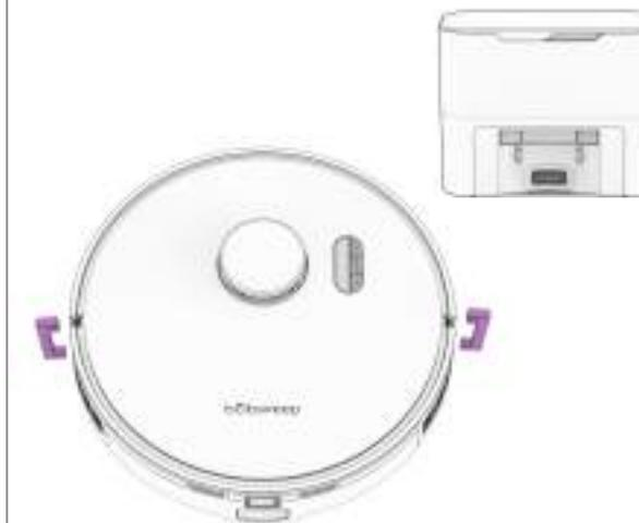
Place the side brush over the empty socket on Orb-i. Press down to click and lock in place.
