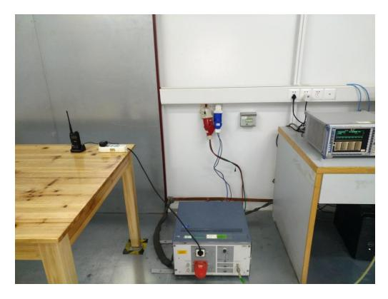
RADIATED EMISSION TEST SETUP-BELOW 1GHz
