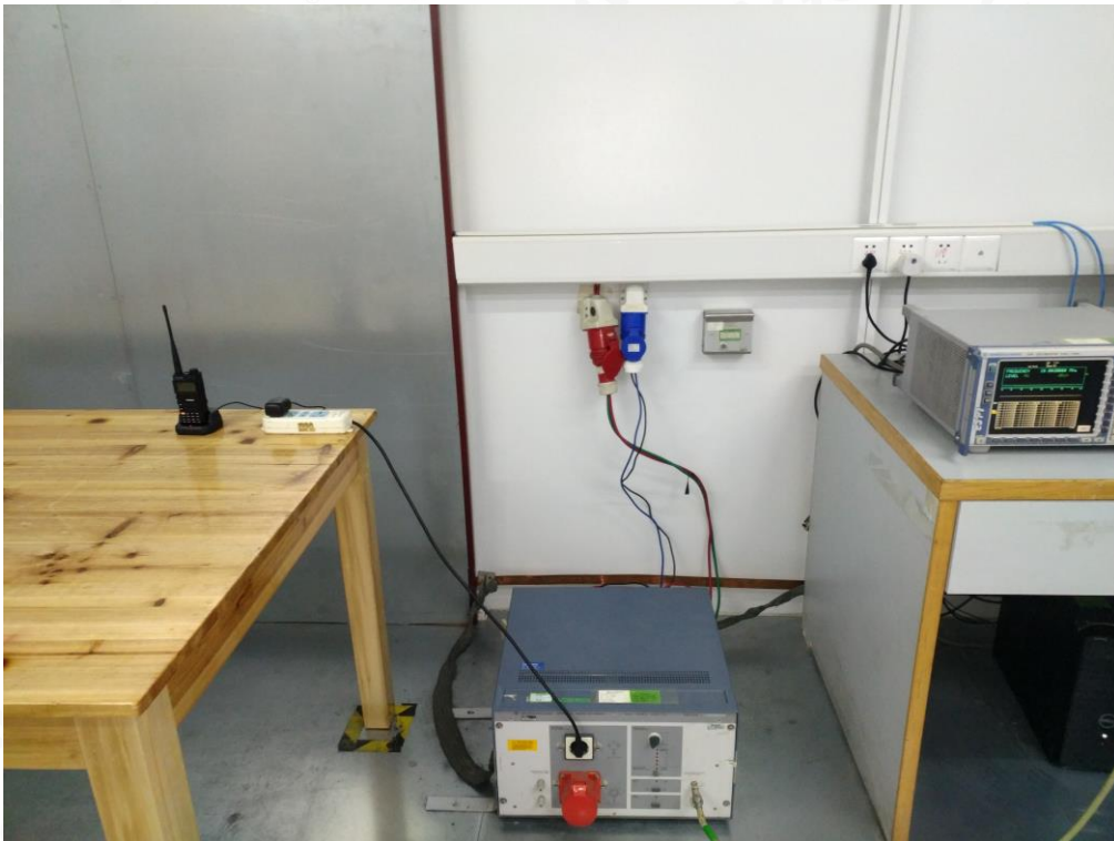
RADIATED EMISSION TEST SETUP-BELOW 1GHZ
