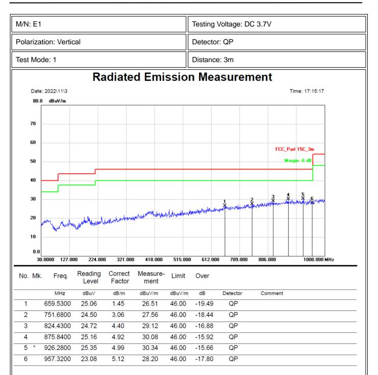
Note: Below 30MHz, the emissions are lower than 20dB below the allowable limit.
