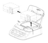
Figure 2-1 Installation Diagram of Label Box
