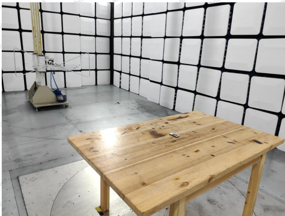
Photo of Radiated Emission Measurement
