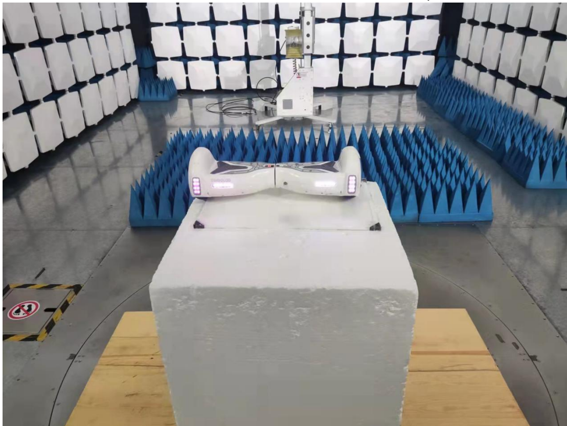
Above 1GHz for radiated emission test setup
