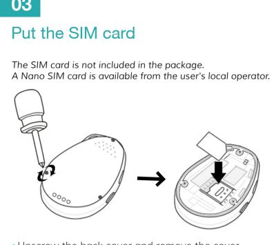
Unscrew the back cover and remove the cover. Insert the SIM card and make sure it's activated with Put the cover back and tighten the screws.
