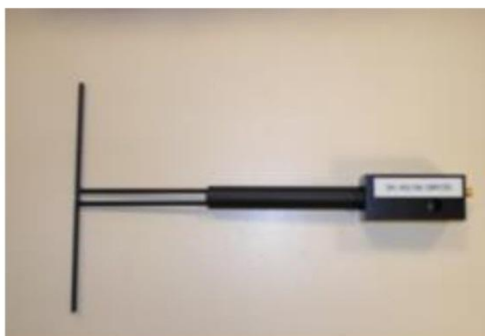
Figure 1 – Satimo COMOSAR Validation Dipole
