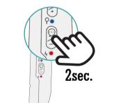
Press and hold button 3 seconds, and in the same time press CALL2 button on charging base, they will pair to each other via bluetooth.
