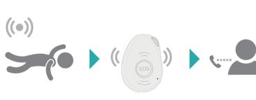
• Due to the daily life activities (like some sports, sit back on a coach, etc), device may detect a fall incorrectly, this situation may cause false alarm. However, users can manually cancel the fall alert by pressing SOS button during its beeping.
