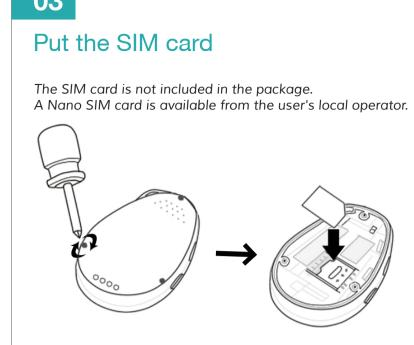
Unscrew the back cover and remove the cover. Insert the SIM card and make sure it's activated with Put the cover back and tighten the screws.
