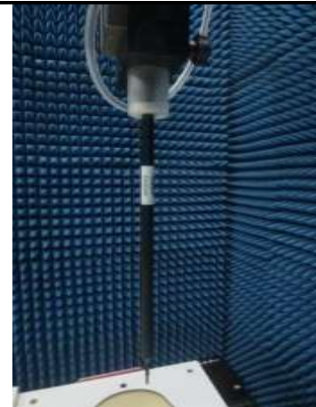
Fig. 8.2 Photo of E-Field Probe
