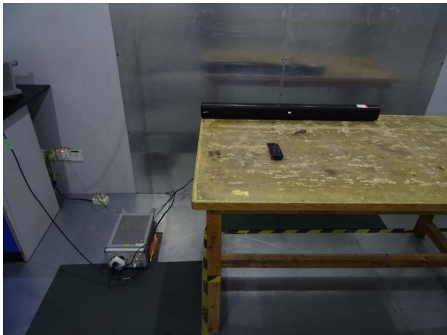
Photograph – Conducted Emission Test Setup
