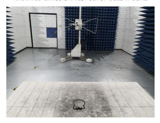
RADIATED EMISSION TEST SETUP ABOVE 1GHZ
