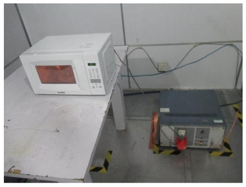
Radiated Emission Test Set-up (30 -1,000MHz):
