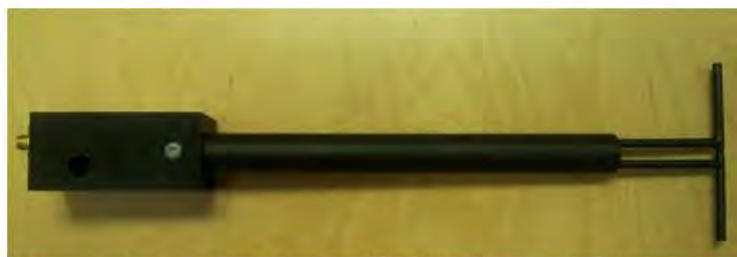
Figure 1 – MVG COMOSAR Validation Dipole
