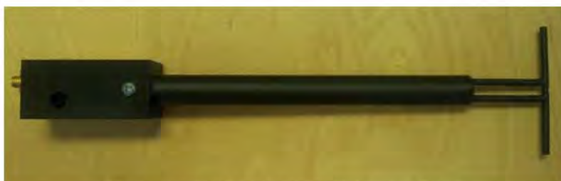
Figure 1 – MVG COMOSAR Validation Dipole
