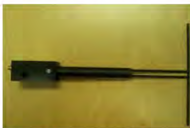
Figure 1 – MVG COMOSAR Validation Dipole
