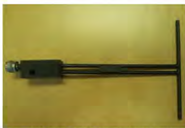
Figure 1 – MVG COMOSAR Validation Dipole
