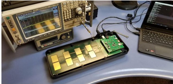
Figure 5: Conducted RF Test Setup Photograph(s).
