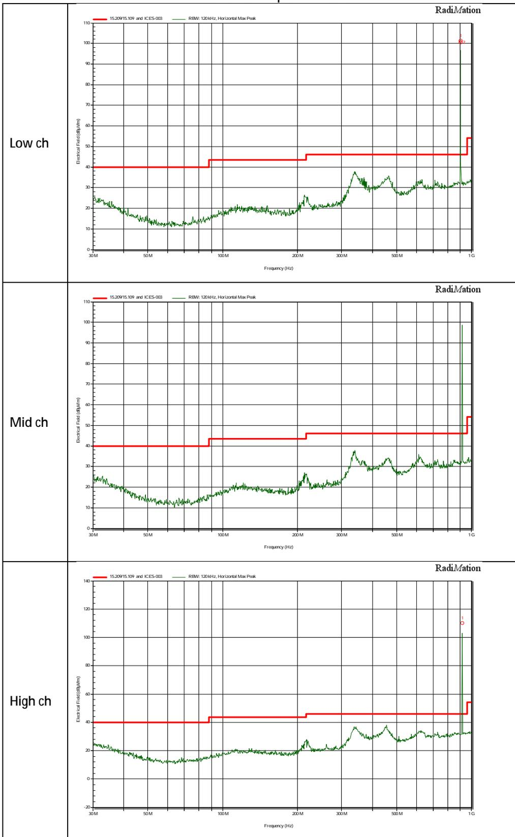
Note: the peak at 900 MHz is the transmission frequency and is not subject to the spurious limit
