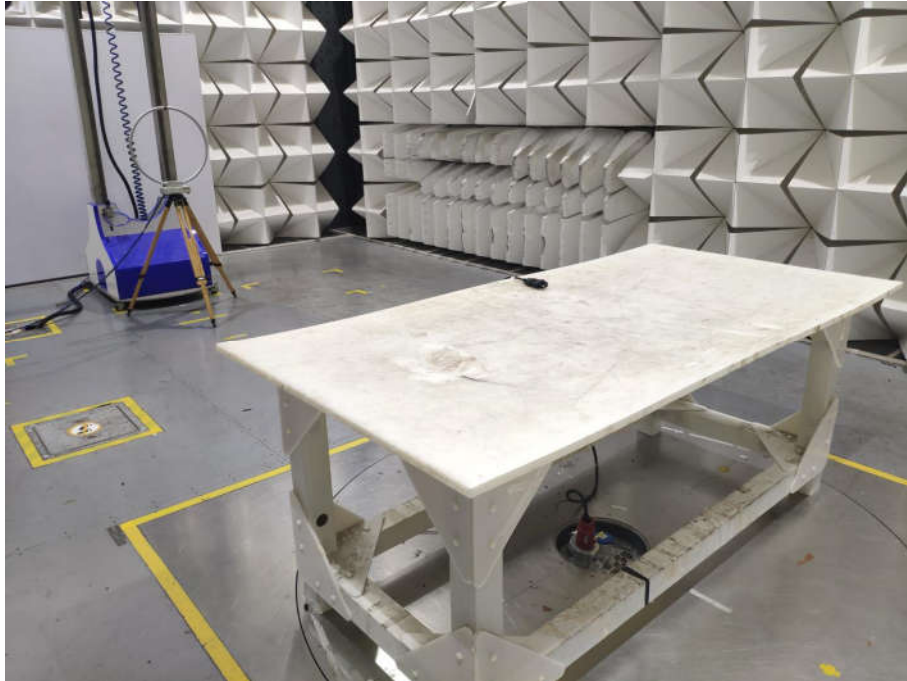
Radiated spurious emission Test Setup-1(Below 30MHz)
