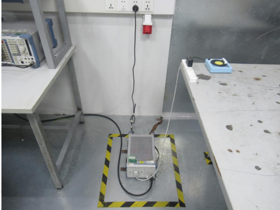
Photo of Conducted Emission Measurement
