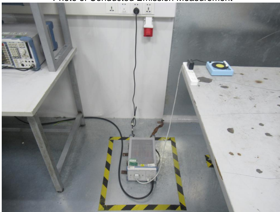
FCC ID: 2AUKG-MLPW Photo of Conducted Emission Measurement
