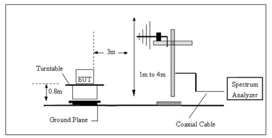
(C) Radiated Emission Test-Up Frequency Above 1GHz
