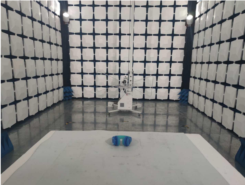
Blow 1GHz for radiated emission test setup
