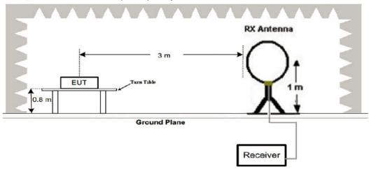
2. Radiated Emission Test-Up Frequency 30MHz~1GHz
