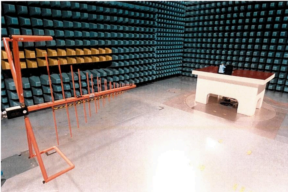
Photo 3: Setup in the Semi anechoic chamber (SAC3) radiated emissions measurement (30 MHz – 1000 MHz)
