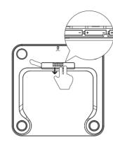
Note: When inserting the batteries, line up the positive and negative signs to make sure the batteries are installed correctly
