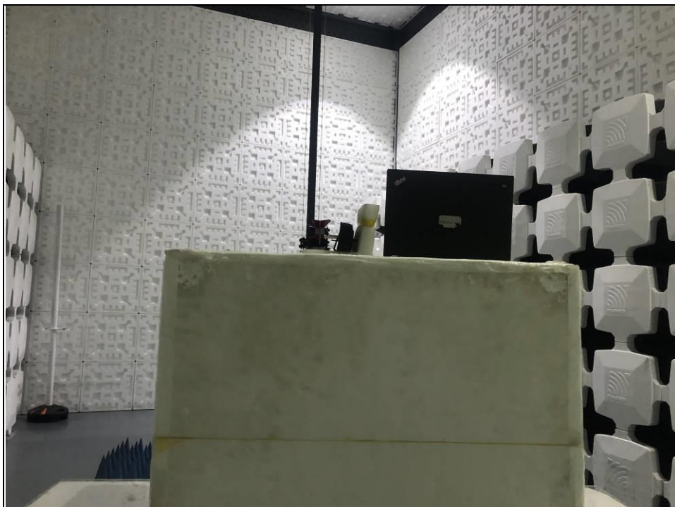
Radiated emission test: Frequency Range < Above 1GHz >
