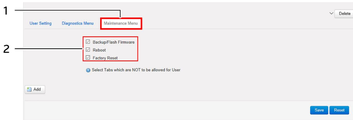
Figure 51: User configuration screen to further manage the user access to maintenance screen options
