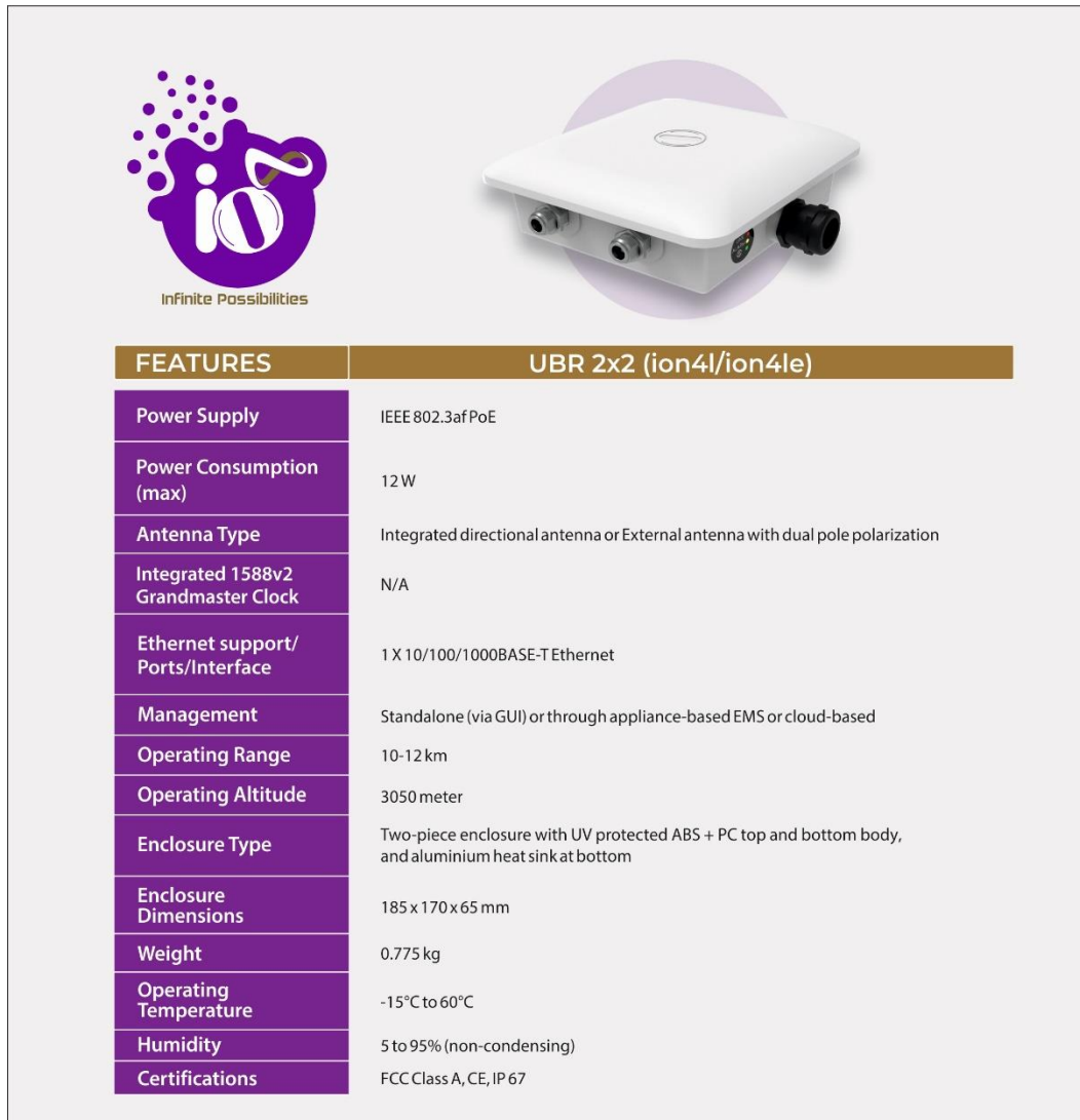
Figure 2: UBR with integrated/external antennas - Specifications & Highlights-2
