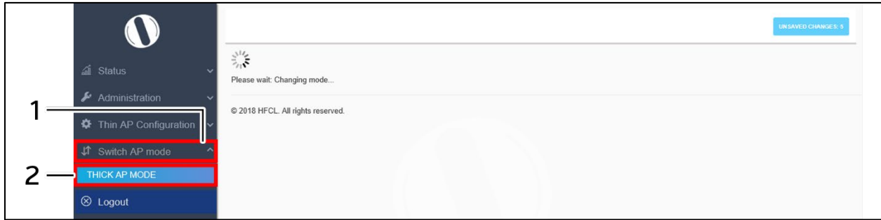
Figure 17: Basic overview of the screen to switch mode from thin AP to thick AP
