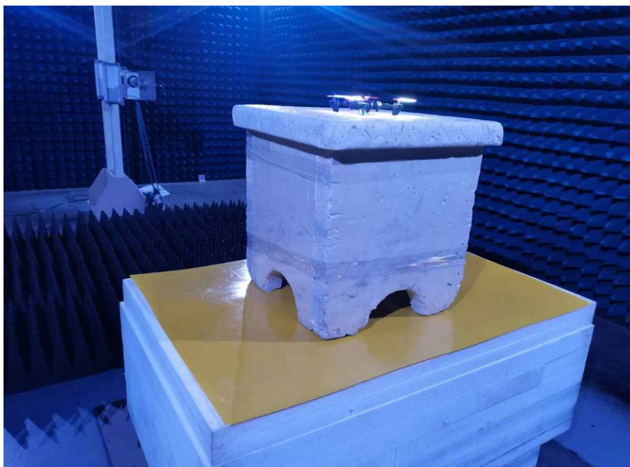
Photo of Radiated Emission Measurement (Above 1G)
