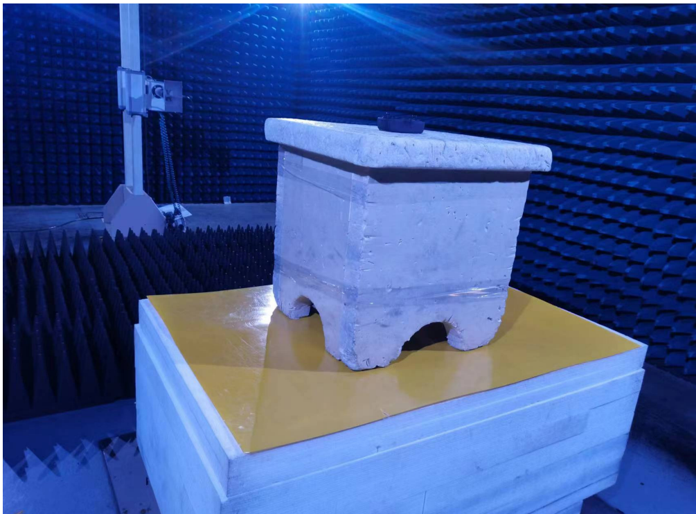
Photo of Radiated Emission Measurement (Above 1G)
