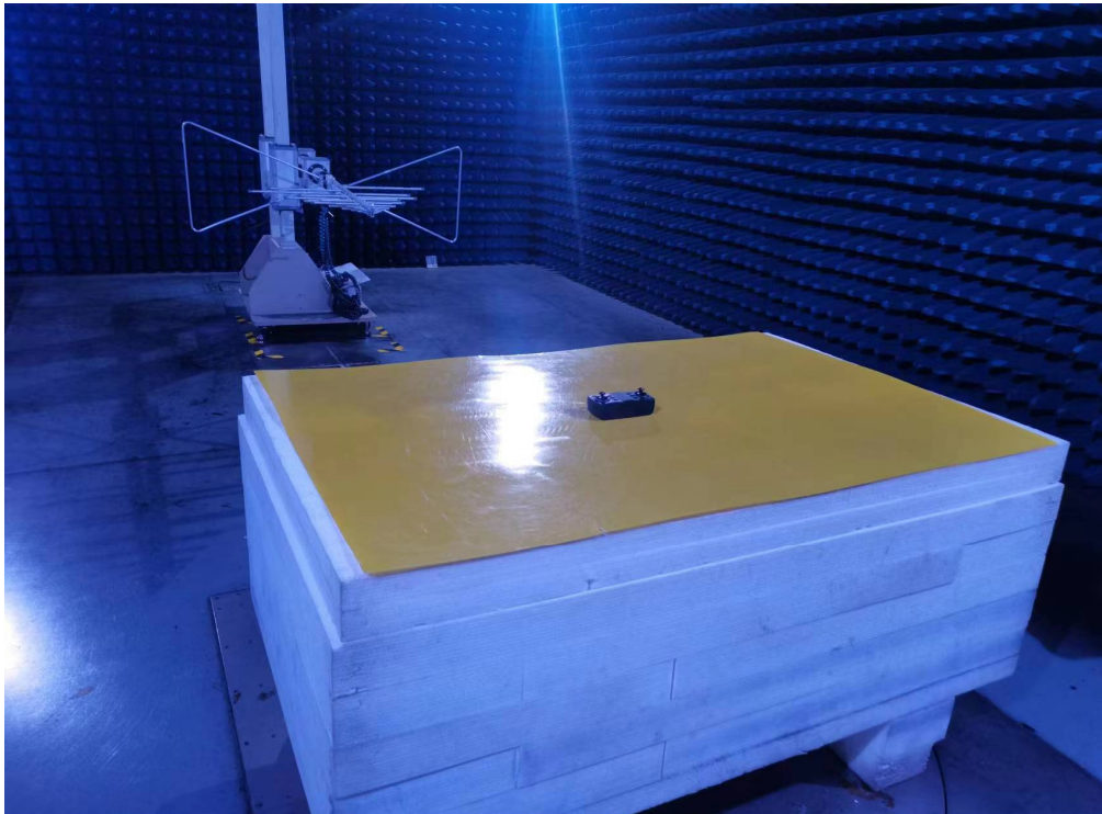
Photo of Radiated Emission Measurement (Above 1G)
