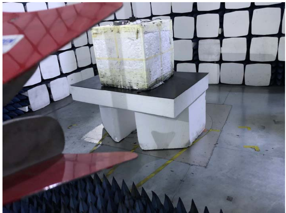
Radiation Emission Test Setup (1GHz to 18GHz)
