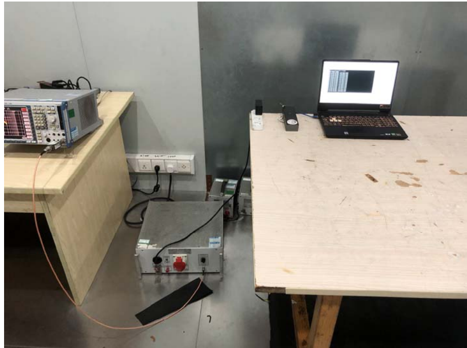
Conducted Emission Test Setup
