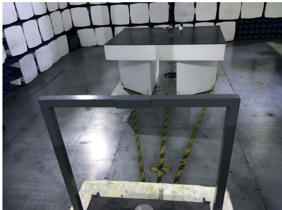
Radiation Emission Test Setup (Below 30MHz)
