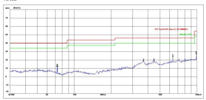
Site: Antenna::Vertical Temperature(C):23.7(C) Limit: FCC Part15 RE-Class B\_30-1000MHz Humidity(%):53.8%
