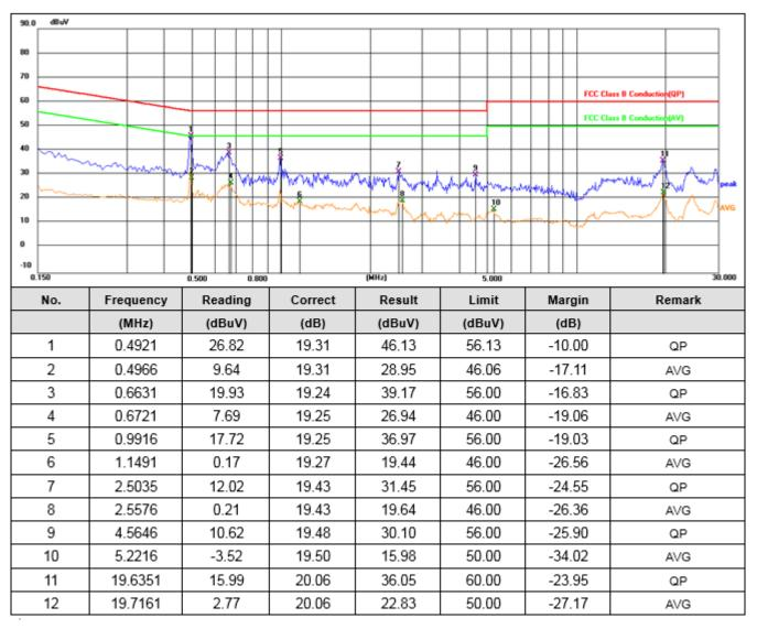
AC Conducted Emission of adapter mode @ AC 120V/60Hz @ (IEEE 802.11n40 mode) (worst case) Line
