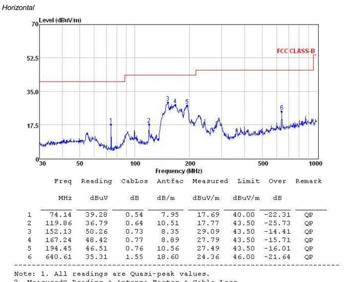
2. Measured= Reading + Antenna Factor + Cable Loss
