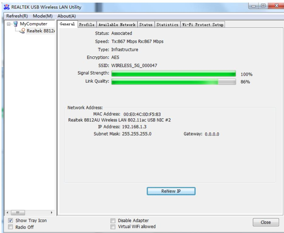
**NOTE:** If you connected to an access point but the connection has been dropped soon, please check security settings and re-check password spelling.
