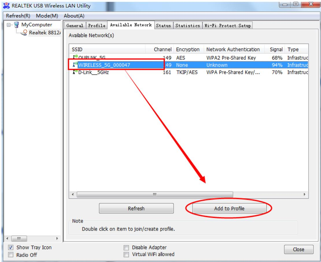
If the wireless access point you wish to connect does not appear here, you can click '**Refresh**' button to scan for wireless access points again; if the wireless access point you're looking for still not appear, try to move the computer closer.
