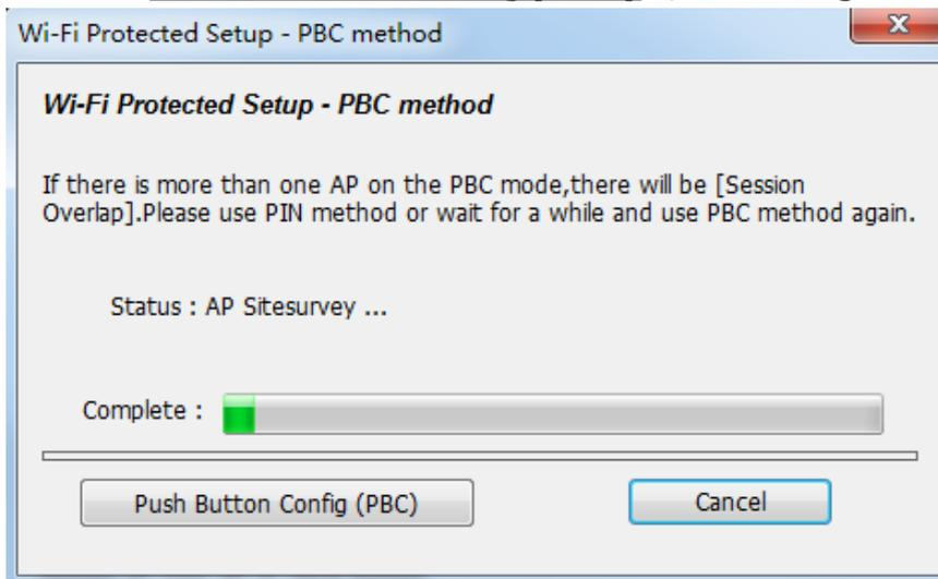
Please activate Push-Button function on wireless access point now, and wireless network card will establish secure connection with access point within one minute.
