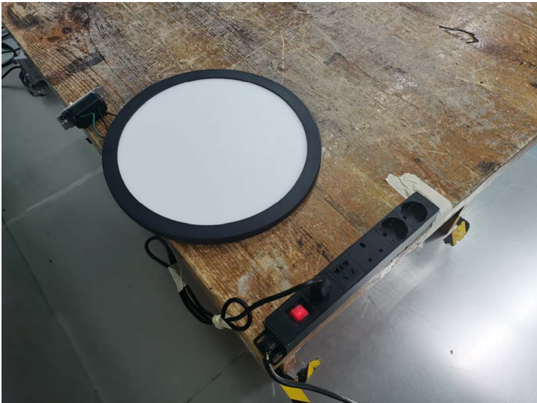
Conducted Emissions Side View
