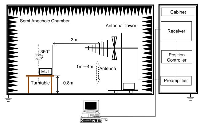
(b) Radiated Disturbance Test Set-Up Frequency above 1GHz
