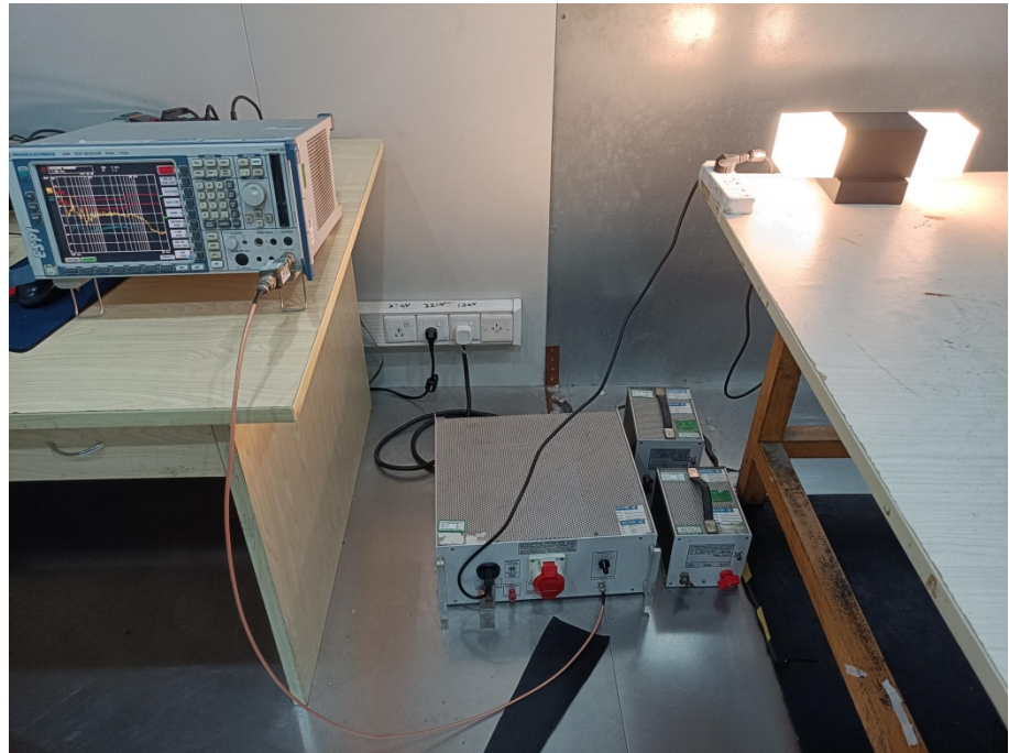
Conducted Emission Test Setup
