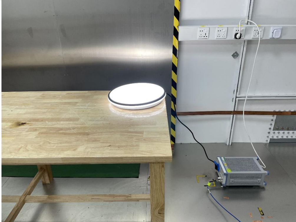
AC Power Line Conducted Emission
