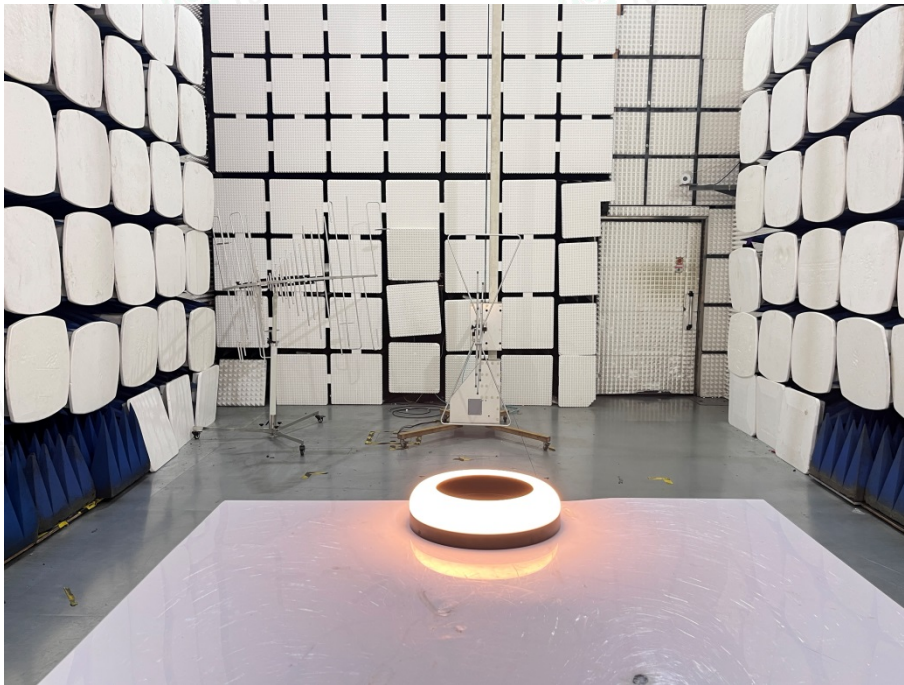
Radiated emissions (Below 1GHz)
