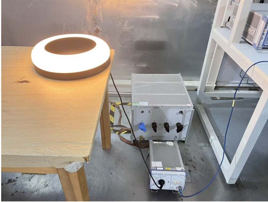
Conducted emissions on AC mains
