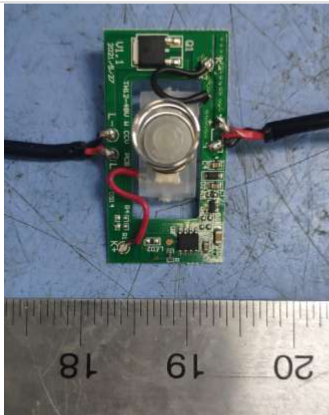
Dimmer PCB View
