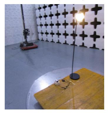
Remark: The EUT is center on the turntable, due to the edge of desk placed on the diameter of the turntable.
